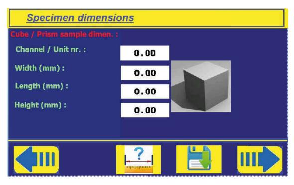
After a short period of time numune Receiving sample information lanmış message is displayed, the predefined sample sizes of this test method are loaded from memory. Thus, the loss of time from entering the same information is prevented.
